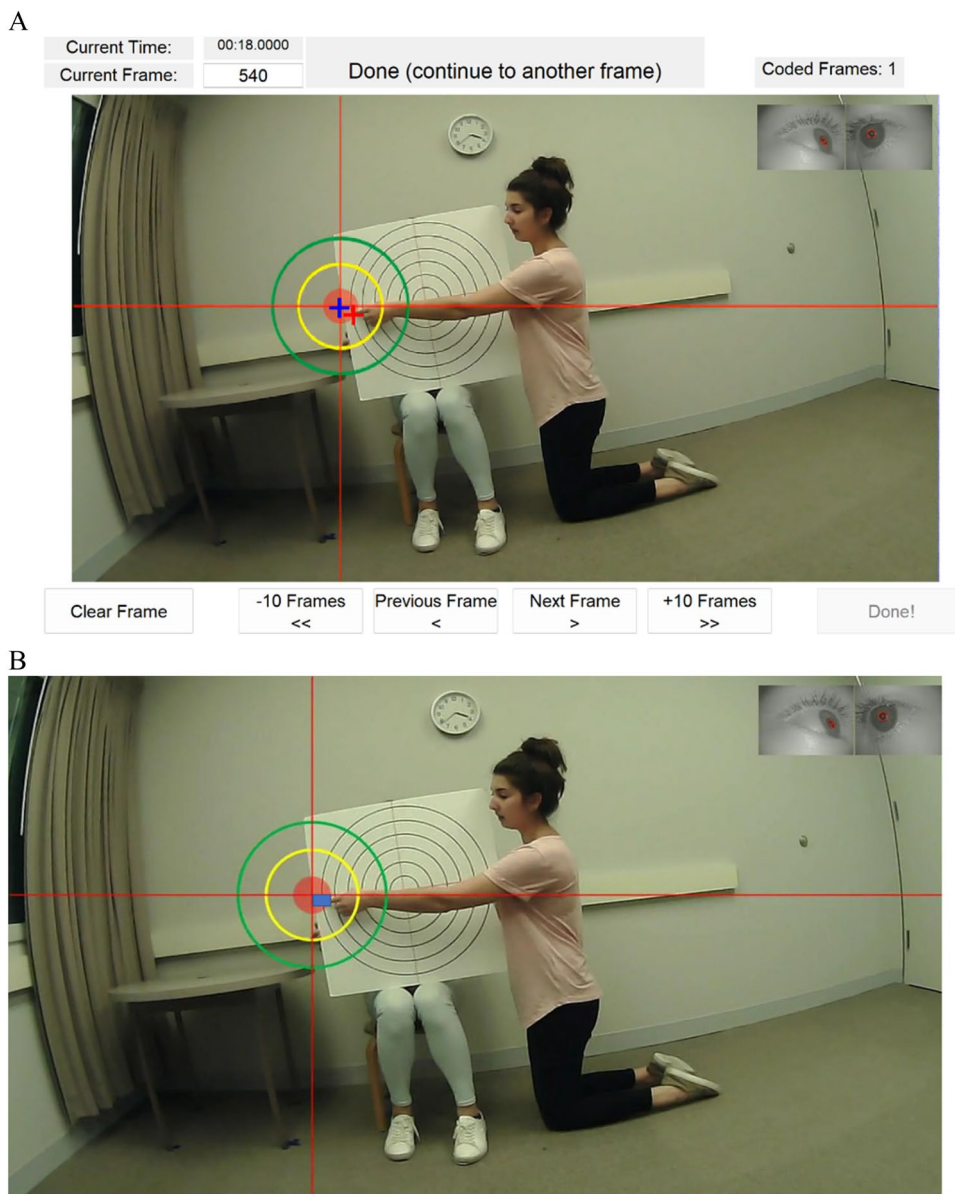
Fig. 1 Screenshots of the graphical user interfaces (GUIs) for accuracy calculation. Both the MATLAB tool (A) and R Shiny app (B) enable users to annotate the point of gaze (i.e., crosshair) and the target location (i.e., where the experimenter is pointing). The data are then used to compute the spatial offset (in degree of visual angle) between the gaze location and the target location. A The MATLAB tool takes video inputs. In this example, 25 frames from the validation session were used for the calculation of accuracy. Based on the
